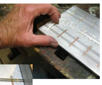
The more distant photo shows that rails are held in place using point forming tools (a conveinient heavy object with a flat bottom).
