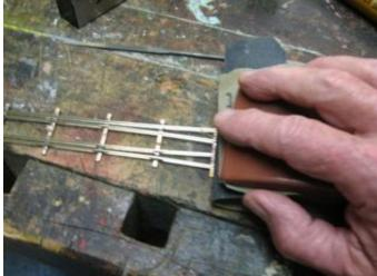
I polished the rail top with a very fine emery cloth before going any further. Then, washed the product with a bit of borax in solution then rinsed the result in warm water. The idea is to reduce corrosion.
