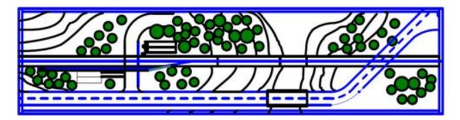
This is an overview of the module that is 2 feet wide and 8 feet long with the main line down the center. The railroad stays level while the land around the tracks undulates up and down. Fills and cuts were used by the railroad to keep the track level, however there are some grades on this line between Rhinelander and Bradley Junction. For the module I have kept the track level.
