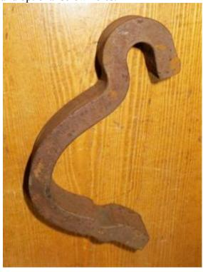
Rail anchors are used to keep the tie from moving along the rail. There are several types (Channel Lock, Drive-On: Unit Wrench: and Unit Drive-On.). The unit wrench type is a simple clamp on design shown on the left (and in the first picture as well) that finds common appplication at turn outs and curves beginning with the lead in: essentially any point where side thrust is expected.
